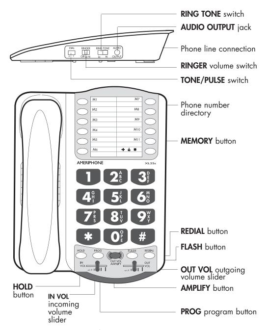
Figure 2 - Base Unit Controls
